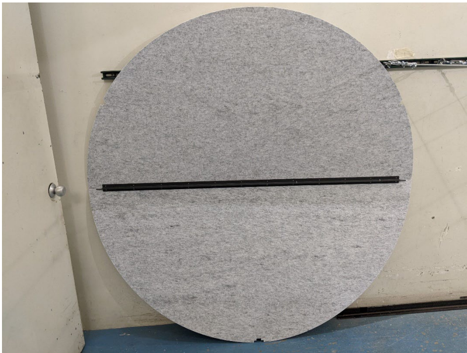
Figure 2 – Individual specimen baffle
