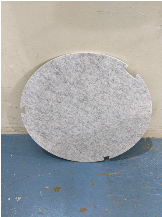
Figure 2 – Individual specimen baffle
